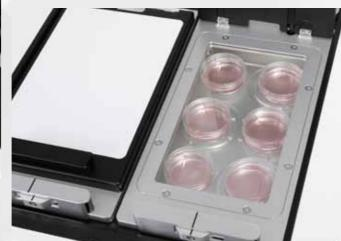
Each Chamber comes with a UNIQUE observation window allowing easy access to the embryo without disturbing it's environment.
