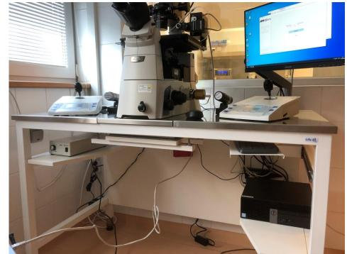
LifeM antivibration tables for micromanipulation workstations with a floating island for the microscope based on an active or pasive AV device from K&S Advanced Systems.
